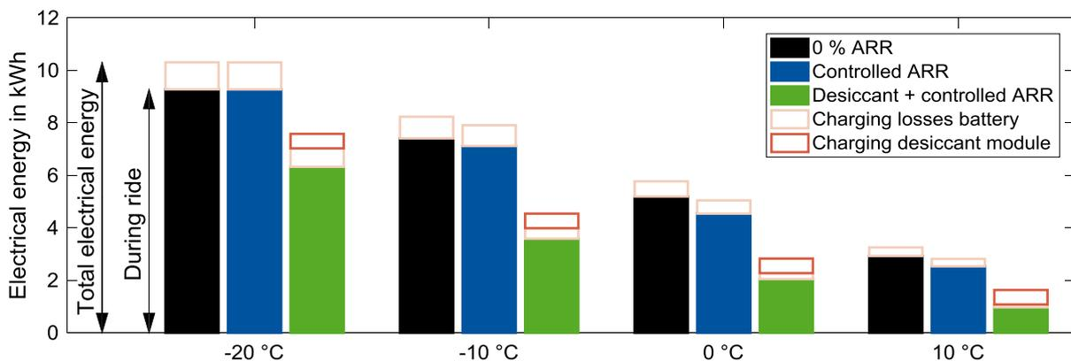
Fig. 4: Electrical energy demand for a 2 h ride at varying ambient temperatures for the three operating strategies: (1) reference strategy with 0 % air recirculation rate (ARR), (2) controlled air recirculation rate, and (3) desiccant-assisted controlled air recirculation rate. The additional electrical energy demand due to charging of the battery and the electrical energy demand for charging the desiccant module are also shown.
