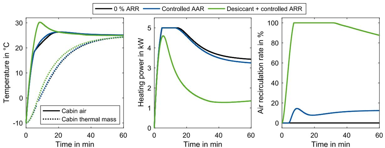
Fig. 6: Transient analysis for outdoor temperature of  $-10\text{ }^{\circ}\text{C}$ : Left: Temperature of cabin air and cabin thermal mass; Middle: Heating power to reach and hold set temperature of  $T_{\text{set,cabin}} = 25\text{ }^{\circ}\text{C}$ ; Right: air recirculation rate while ensuring  $\varphi_{\text{windshield}} < 80\text{ }%$ .
