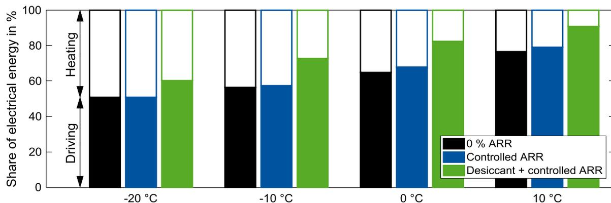
Fig. 5: Share of electrical energy used for driving/heating at varying ambient temperatures for the three operating strategies: (1) reference strategy with 0 % air recirculation rate (ARR), (2) controlled air recirculation rate, and (3) desiccant-assisted controlled air recirculation rate.
