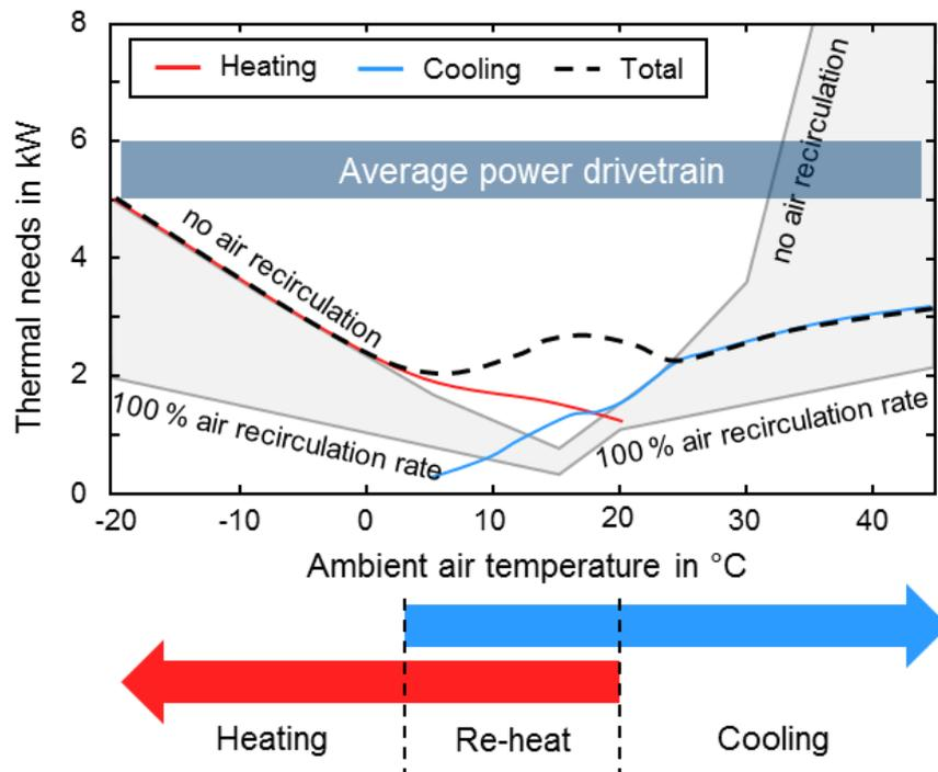
Fig. 1: Top: Energy demand for HVAC system and drivetrain: The energy demand for the HVAC system is based on a simulation study by Brèque and Nemer [10]. The average power for the drivetrain is derived from measurement data reported by Tober [4]. Bottom: Overview on heating and cooling modes based on ambient temperatures [18].
